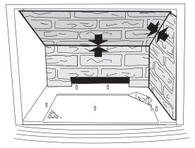
Figure 42. Install Upper Rear Panel
